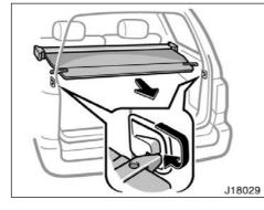
To use the luggage cover, pull it out of the retractor and hook it to the anchors.
