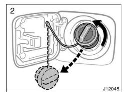
2. To remove the fuel tank cap, turn the cap slowly counterclockwise, then pause slightly before removing it.
