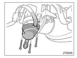
1. Loosen the cover retaining screws and remove the cover.
