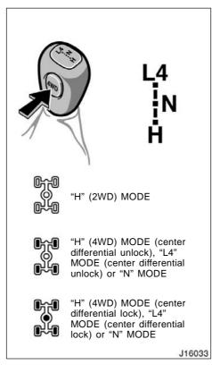
Use the front drive control lever, "4WD" button and center differential lock switch to select the transfer and center differential modes.
