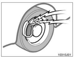
The brake pad wear limit indicators on your disc brakes give a warning noise when the brake pads are worn to where replacement is required.
