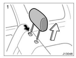
TO USE OUTSIDE ANCHOR BRACKET: 1. Remove the head restraint.
