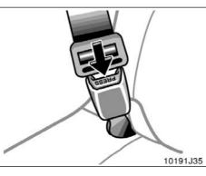
3. To remove the convertible seat, press the buckle-release button.
