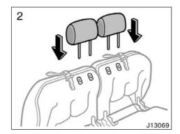
2. Store the head restraints in the head restraint retaining holes in the bottom cushion.
