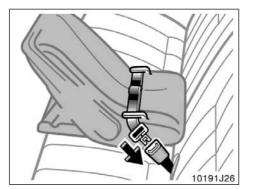
1. Run the center lap belt through or around the infant seat following the instructions provided by its manufacturer and insert the tab into the buckle taking care not to twist the lap belt.
