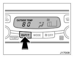
The thermometer indicates the outside air temperature when you push the "OUT/T" button.
