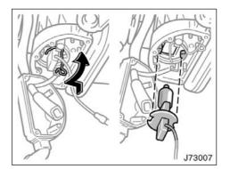
3. Release the bulb retaining spring and remove the bulb. Install a new bulb and the bulb retaining spring.
