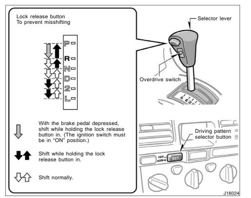
Your automatic transmission has a shift lock system to minimize the possibility of incorrect operation. This means you can only shift out of "P" position when the brake pedal is depressed (with the ignition switch in "ON" position and the lock release button depressed).
