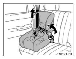
3. While pressing the convertible seat firmly against the seat cushion and seatback, let the shoulder belt retract as far as it will go to hold the convertible seat securely.
