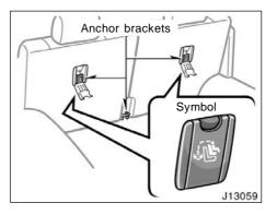
Use the anchor bracket on the back of the rear seatback to attach the top strap.
