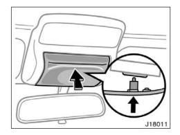
When the garage door opener transmitter is properly installed, you can operate the transmitter by pushing the cover.
