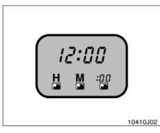
If the electrical power source has been disconnected from the clock, the time display will automatically be set to 1:00 (one o'clock).
