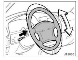
To change the steering wheel angle, hold the steering wheel, pull the lock release lever toward you, tilt the steering wheel to the desired angle and return the lever to its original position.
