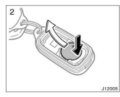
2. Remove the discharged transmitter battery.
