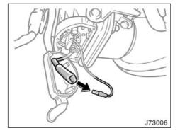
2. Lift up the soft casing and disconnect the cords.
