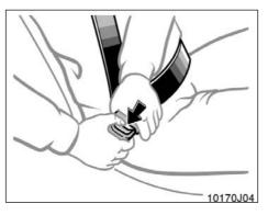
To release the belt, press the buckle-release button and allow the belt to retract.
