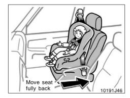
à A forward-facing child restraint system should be allowed to be installed on the front passenger seat only when it is unavoidable. Always move the seat as far back as possible, because the force of the deploying front passenger airbag could cause death or serious injury to the child.
