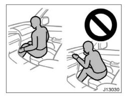
à Do not sit on the edge of the seat or lean over the dashboard when the vehicle is in use. The airbags inflate with considerable speed and force; you may be killed or seriously injured. Sit up straight and well back in the seat, and always use your seat belt properly.
