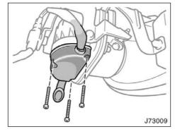
5. Install the cover with the retaining screws.
