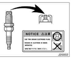
Your engine is fitted with twin ground electrode spark plugs.
