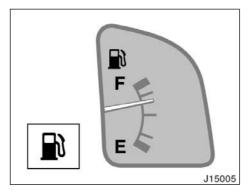
If the fuel tank is completely empty, the malfunction indicator lamp comes on. Fill the fuel tank immediately.
