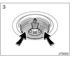
3. Install the rubber cover with the "TOP" mark upward and snuggle on the boss. Plug in the connector.
