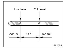
With the engine at operating temperature and turned off, check the oil level on the dipstick.
