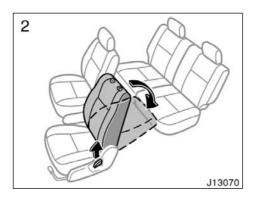
2. Pull the lock release lever up, then push down the seatback.
