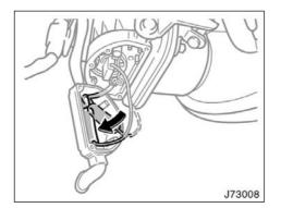
4. Connect the cord and put the soft casing into the cover.
