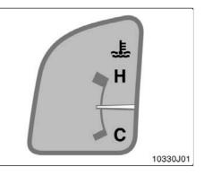
The gauge indicates the engine coolant temperature when the ignition switch is on. The engine operating temperature will vary with changes in weather and engine load.
