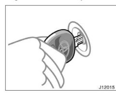
The engine immobiliser system is a theft prevention system. When you insert the key in the ignition switch, the transponder chip in the key's head transmits an electronic code to the vehicle. The engine will start, only when the electronic code in the chip corresponds to the registered ID code for the vehicle.
