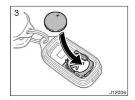
3. Put new transmitter battery with positive (+) side up.
