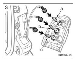
a: Back–up light b: Rear turn signal lights c: Stop/tail light
