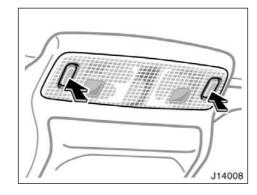
To turn on the personal light, push the switch. To turn the lights off, push the switch once again. Luggage compartment light
