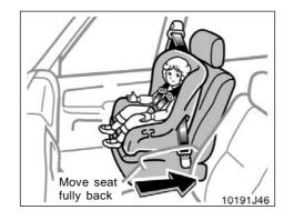
à A forward-facing child restraint system should be allowed to be installed on the front passenger seat only when it is unavoidable. Always move the seat as far back as possible, because the force of the deploying front passenger airbag could cause death or serious injury to the child. For instructions concerning the installation of a child restraint system, see "Child restraint" in this section.
