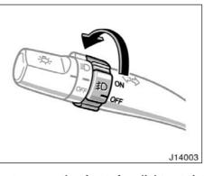
To turn on the front fog lights, twist the band of the headlight and turn signal switch lever. They will come on only when the headlights are on low beam. Interior light
