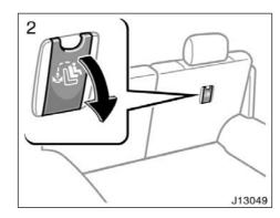
2. Open the anchor bracket cover with the symbol mark shown in the illustration.
