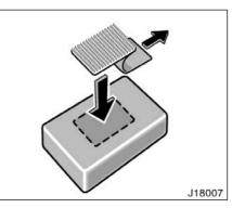
Remove the paper strip covering the adhesive on back side of loop and adhere loop to back side of the transmitter near center.
