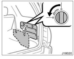
To open the box, turn the two knobs.
