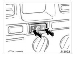
The back window can be operated with the inner switch on the center console or outer switch on the back door.
