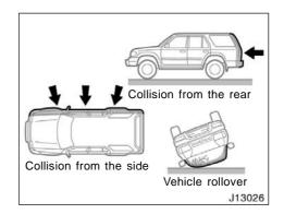
The SRS airbags are not designed to inflate if the vehicle is involved in a side or rear collision, if it rolls over, or if it is involved in a low-speed frontal collision.
